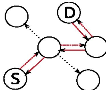
Gambar 3 AODV Routing
