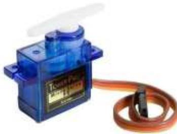
Gambar 2. 11 Motor Servo (Rayhan Al Hayubi et al., 2024).
