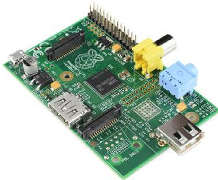
Gambar 2.8 *Raspberry Pi Model A*
