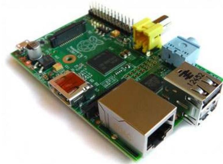
Gambar 2.10 Raspberry Pi Model B
